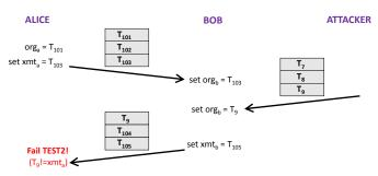
Fig. 11. Alice (left) exchanges symmetric mode packets with Bob (center). Attacker (right) is *on-path* for authenticated NTP and *off-path* for unauthenticated NTP. For the on-path authenticated DoS attack, the attacker's packet (timestamps  $T_7$ ,  $T_8$ ,  $T_9$ ) is a replay of a stale packet sent from Alice to Bob. For the off-path unauthenticated DoS attack, the attacker's packet is spoofed.
