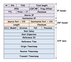
Fig. 1. NTP mode 4 server response packet. (Client queries have the same format, but with mode field set to 3. Symmetric mode uses mode 1 or 2. Broadcast mode uses mode 5).
