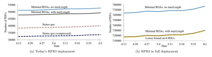
Figure 3: Number of PDUs processed by routers under different scenarios along a timeline. A solid line marks scenarios that are safe against forge-origin subprefix hijacks. Scenarios with dashed lines are vulnerable.
