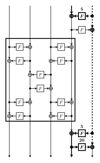
Fig. 14. A differential characteristic for (reduced-round) Simpira with b = 5 that has 30 active S-boxes. A thick full line indicates a difference in every byte, a thick dotted line refers to a difference in only one byte – it does not matter which one. A normal line indicates that no difference is present. When non-zero, the number of active S-boxes is shown above every F-function.
