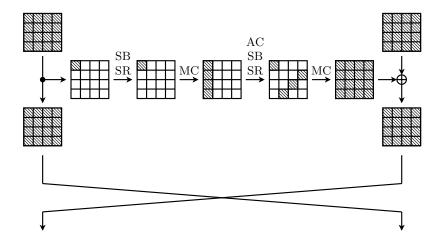
**Fig. 5.** A linear characteristic for one round of Simpira with b = 2 with 5 active Sboxes. Crosshatches represent bytes with non-zero linear masks. As Simpira uses two AES rounds per *F*-function, it can reach 25 active S-boxes in only 5 Feistel rounds, corresponding to 10 AES rounds in total.
