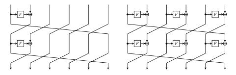
Fig. 1. Two common classes of Generalized Feistel Structures (GFSs) are the Type-1 GFS (left) and the Type-2 GFS (right). For each example, two rounds are shown of a GFS that operates on b = 6 subblocks. We will initially consider these GFSs in this paper, as well as other GFSs with a different number of *F*-functions per round, and other *subblock shuffles* at the end of every round. At a later stage, we will consider more advanced constructions as well.
