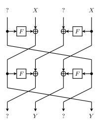
**Fig. 13.** Yanagihara and Iwata Type-1.x (4,2) GFS [80], which was used in Simpira v1 for b = 4. Here '?' is a wildcard character that can represent any value. Also X can correspond to any value, but both occurences of X must correspond to the same value. The leftmost input subblock enters the same F-function twice, and therefore guarantees that the output value Y will appear twice as well.
