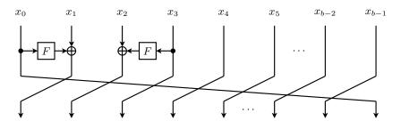
**Fig. 12.** Yanagihara and Iwata's Type-1.x (b,2) GFS [80], which was used in Simpira v1. Note that regardless of b, the same  $x_0$  will eventually enter an F-function twice after a sufficient number of rounds.
