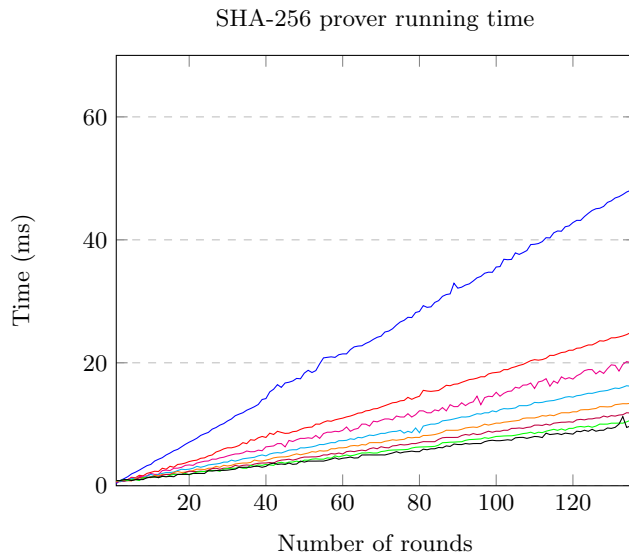
Fig. 8. Relation between the running time ( without disk reading operations ) and the number of rounds for the SHA-256 prover, average over 100 runs.
