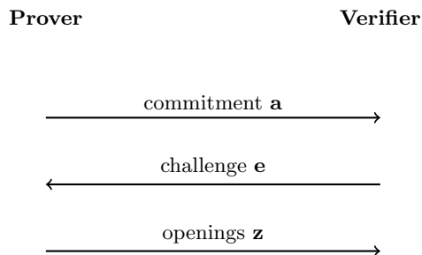
Fig. 1. The communication pattern of a \Sigma -protocol.
