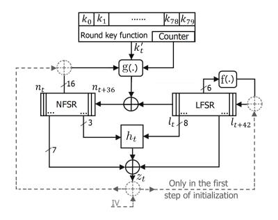
Figure 1: The Block Diagram of Fruit
