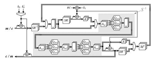
Fig. 5. Round-based first-order threshold implementation of PRINCE
