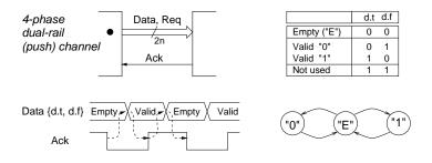
Fig. 9. A delay-insensitive 4-phase dual-rail protocol (taken from [45])
