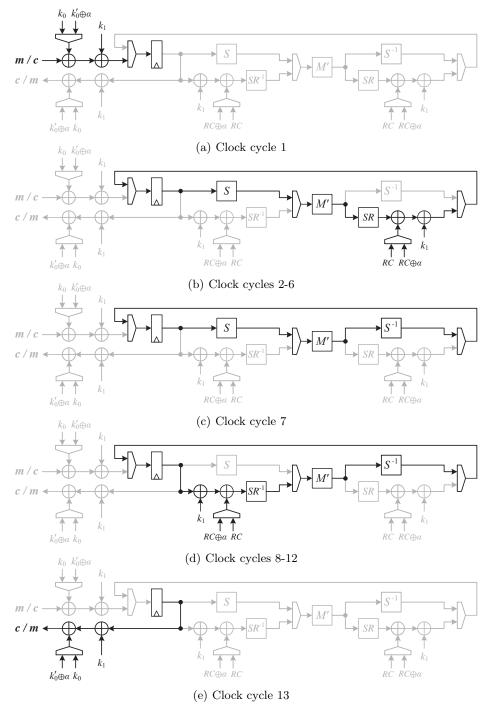
Fig. 17. Detailed active parts of the original round-based architecture [13]
