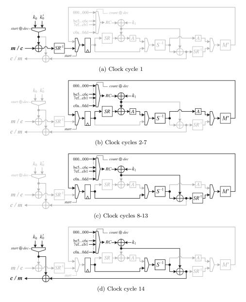
Fig. 18. Detailed active parts of our round-based architecture
