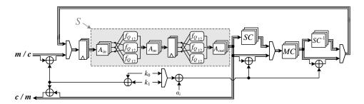
Fig. 15. Round-based first-order threshold implementation of Midori64
