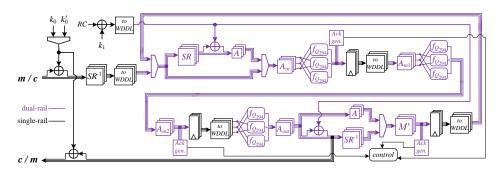
Fig. 11. Asynchronous round-based first-order threshold implementation of PRINCE
