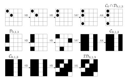
**Figure 9:** 3-rounds Truncated Differential Attack on AES with a single secret S-Box. The choice of the plaintexts (i.e.  $p_{0,0} \oplus p_{1,1} = k_{0,0} \oplus k_{1,1}$ ) guarantees that after one round there are only three bytes with non-zero difference instead of four, that is the plaintexts belong to the same coset of  $C_0 \cap D_{0,1,3}$ . White box denotes denotes a byte with a zero-difference, while a black box denotes a byte with non-zero difference.
