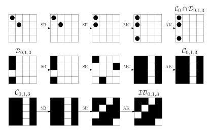
**Figure 13:** 3-round Truncated Differential Attack on AES with secret S-Box. The choice of the plaintexts (i.e.  $p_{0,0} \oplus p_{1,1} = k_{0,0} \oplus k_{1,1}$ ) guarantees that after one round there are only three bytes with non-zero difference instead of four, that is the plaintexts belong to the same coset of  $C_0 \cap D_{0,1,3}$ . White box denotes denotes a byte with a zero-difference, while a black box denotes a byte with non-zero difference.
