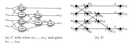
Figure 1: A 2-bit adder circuit C and corresponding circuit DAG D.
