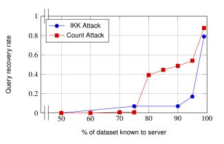
Figure 6: Query recovery rates when server has partial knowledge of true document set. Enron dataset, 500 keywords, 150 queried uniformly.
