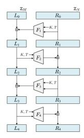
Figure 3: On the left is code for the encryption and decryption algorithms of  $F = \mathbf{Feistel}[r, M, N, \boxplus, \mathrm{PL}]$ , where  $\mathrm{PL} = (\mathcal{T}, \mathcal{K}, F_1, \dots, F_r)$ . On the right is an illustration of encryption with r = 4 rounds.
