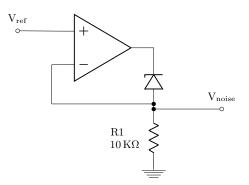
Figure 5: Bias circuit for an avalanche diode.
