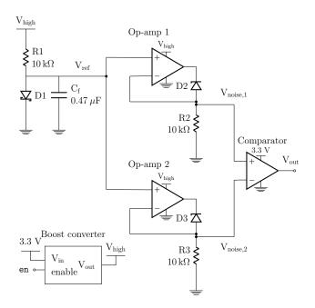
Figure 9: The Lampert circuit. The boost converter is shown in Figure 7. A microcontroller controls the boost converter and samples bits from  $V_{\rm out}$  (§3.5).
