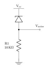
Figure 2: Avalanche noise test circuit.
