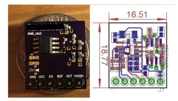
Figure 10: Standalone RNG board. On the left is final design over a US quarter; on the right is the printed circuit board layout with dimensions in mm.
