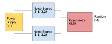
Figure 1: Block diagram of the Lampert circuit. Random bits are sampled from the comparison between two noise sources.
