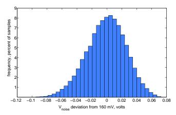
Figure 4: Histogram of deviation of  $V_{\text{noise}}$  from 160 mV for the test setup in Figure 2,  $V_{cc} = 12.16$  V, for 500 000 samples taken at 1 ns intervals.
