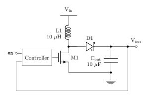
Figure 7: A boost converter takes a DC input voltage,  $V_{in}$ , and produces a higher DC output voltage,  $V_{out}$  (§3.4). The circuit is enabled via the logic-level en input. In our implementation (§6) the switch (M1) and the controller are integrated into a single chip.
