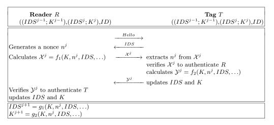
Fig. 5. Generalized ultralightweight mutual authentication protocol (GUMAP)
