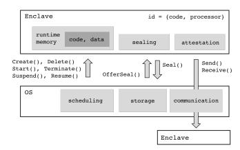
Fig. 1: SGX model. We model enclaves and the operating system, their main functionality, and the operations (scheduling, storage, communication) through which they interact.
