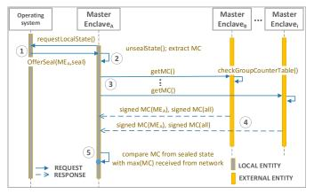
Fig. 6: ME start protocol. The ME obtains the latest MC value from the assisting MEs and verifies the integrity of the unsealed data using it.
