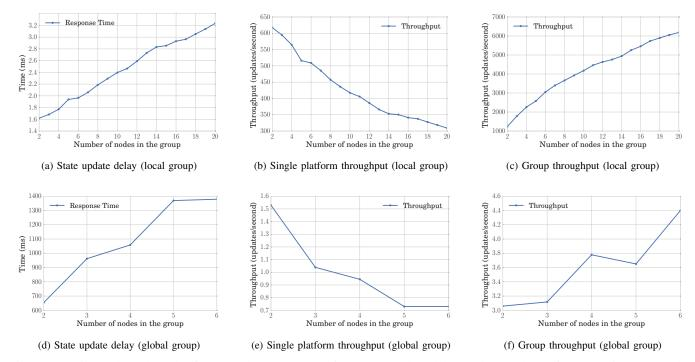
Fig. 9: Experimental results. The first row shows ROTE performance (update delay and throughput) for protection groups that are connected over a local network. The second row show performance for geographically distributed protection groups.
