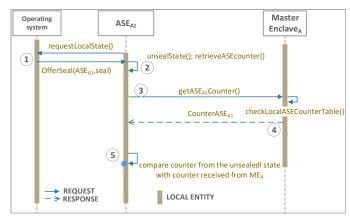
Fig. 5: ASE start protocol. An ASE obtains the latest data state counter from the ME and verifies the integrity of the unsealed data using it.
