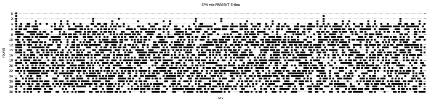
Figure 7. Differential behavior of an SP Network Bit-Mixer with the PRESENT Cipher S-Box
