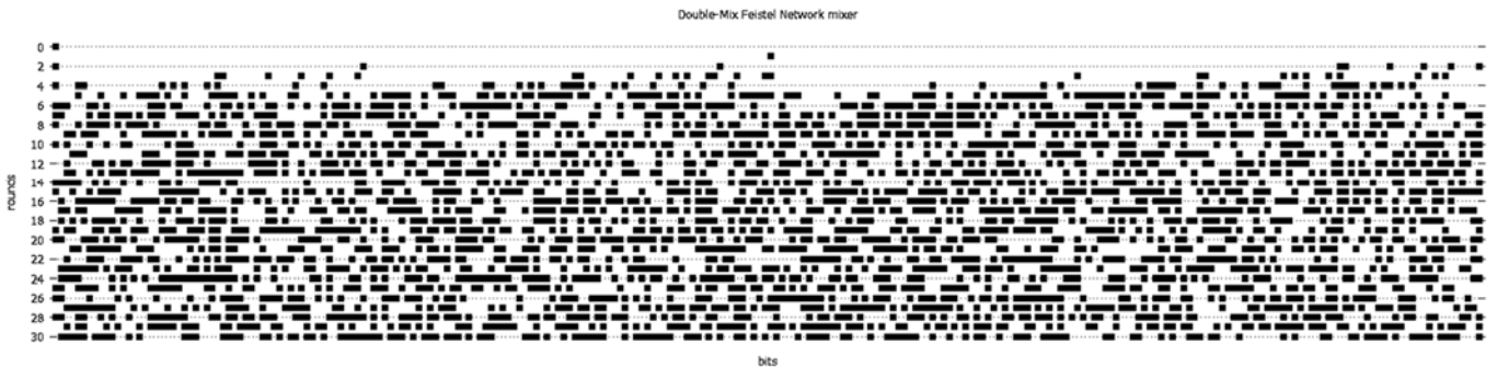
Figure 9. Differential behavior of a DMFN bit-mixer with shift distances: {9, 73, 1, 17, 6, 25, 11, 26}
