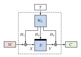
**Fig. 1:** Schematic illustration of the encryption process of a message M and a tweak T with the general  $GXHX[E,\mathcal{H}]$  tweakable block cipher.  $E:\mathcal{K}\times\{0,1\}^n\to\{0,1\}^n$  is a keyed permutation and  $\mathcal{H}:\mathcal{L}\times\mathcal{T}\to\{0,1\}^n\times\mathcal{K}\times\{0,1\}^n$  a keyed universal hash function.
