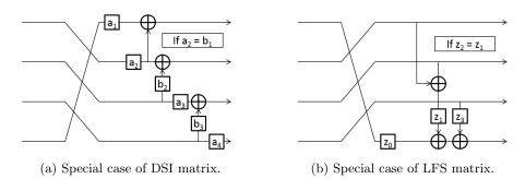
Fig. 3: Saving implementation cost for serial-type matrices.
