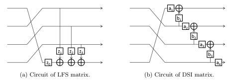
Fig. 2: Circuit of LFS and DSI matrices of order 4.
