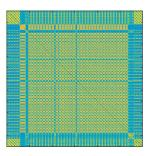
**Fig. 6.** Cross-correlation for SW implementation, d = 3, SubBytes. One can identify the 34 AND gates in the SubBytes circuit of Boyar et al. [11].
