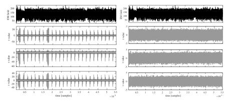
Fig. 4. Non-specific leakage detection on SubBytes. Left column: masks off. Right column: masks on. Rows (top to bottom): one exemplary EM trace, first-order t-test; second-order t-test; third-order t-test. SPA features within an electromagnetic trace are better visible in the cross-correlation matrix shown in Figure 6.
