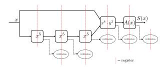
Fig. 2. AES S-box pipeline
