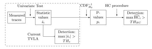
Fig. 2: HC leakage detection flow chart.
