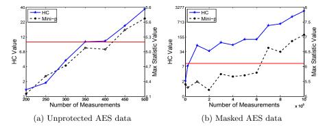
Fig. 5: Statistic Values of Mini-p and HC procedures on two AES implementations.
