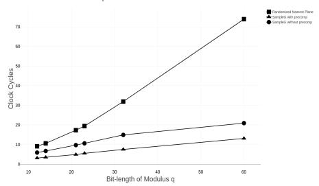
Figure 3: Measured clock cycles with  $q = \{4093, 12289, 1676083, 8383498, 4295967357, \approx 9 \cdot 10^{18}\}$  and s = 100 averaged over 100,000 runs. The clock cycles for the last three moduli are  $\{19.4, 31.9, 73.9\}$  for GPV and  $\{5.5, 7.5, 13.1\}$  for SAMPLEG with pre-computation.
