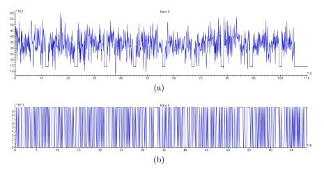
**Fig. 2.** Figure (a) is a typical example of a (hardware) power trace of an unprotected AES-128 implementation (one can observe the ten rounds). Figure (b) is a typical example of a portion of a serialized software trace of stack writes
