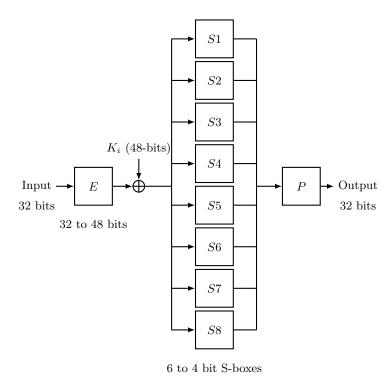
**Fig. 8.** The Feistel function (F) within the DES cipher.
