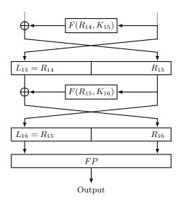
Fig. 7. The final rounds of the DES cipher.
