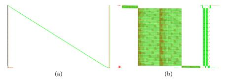
**Fig. 3.** (a) Visualization of a software execution trace of the binary Wyseur white-box challenge showing the entire accessed address range. (b) A zoom on the stack address space from the software trace shown in (a). The 16 rounds of the DES algorithm are clearly visible.
