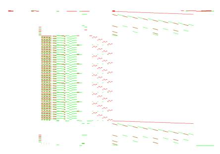
Fig. 6. Visualization of the stack reads and writes in the software execution trace portion limited to the core of the Karroumi WB-AES.
