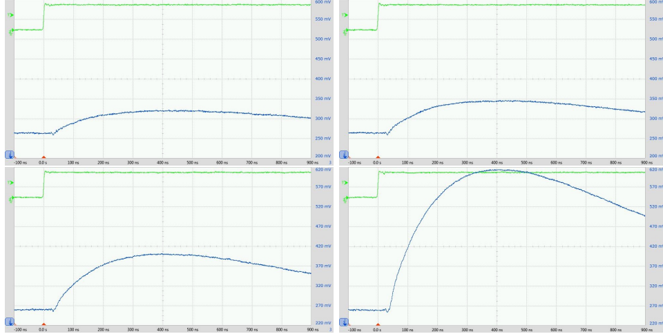
Fig. 1: A picture of a single trace captured for the second cycle of the encryption for SIMON (top) and SPECK (bottom) for d = 4 configurations of 64/128 (left) and 128/128 (right). The clock pulse is shown in green (upper trace in each picture) and the amplified V_{INT} signal is shown in blue. Note how the power consumption with increasing n is substantially greater for SPECK than for SIMON due to the cascading effects of the addition carry. The vertical range showing the raw power measurement is 400mV and the horizontal range is 1\mu s .
