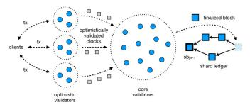
Fig. 4: Trust-but-Verify Validation Architecture
