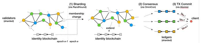
Fig. 2: OmniLedger architecture overview: At the beginning of an epoch e, validators (1) use RandHound to randomly remove old validators from shards and assign new validators who registered to the identity blockchain in epoch e-1. Afterwards, validators ensure (2) consistency of the shards' ledgers via Omnicon while clients ensure (3) consistency of their cross-shard transactions via Atomix (here the client spends inputs from shards 1 and 2 and outputs to shard 3).
