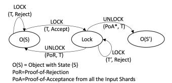
Fig. 16: State-Machine for state-full objects. Pessimistic locking is necessary
