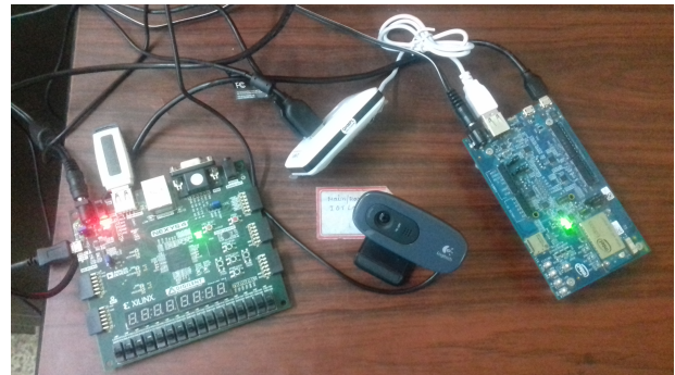
Fig. 8. Experimental setup for smart IoT node.
