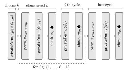
Fig. 6: Protocol to implement a generalized coupled rotation with  $\ell+1$  cycles of length  $t_0, t_1, \ldots, t_{\ell}$ . Notation is explained in the text.
