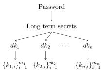
Figure 1: Relationship between secrets (the notation  $a \rightarrow b$  indicates that the value b can only be recovered using the value a).
