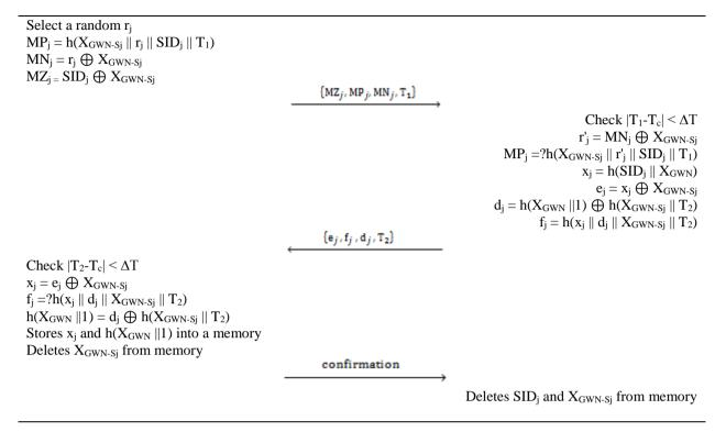
Figure 5. Sensor node registration phase of the proposed scheme.
