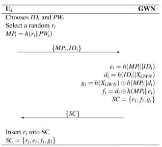
Figure 1. User Registration phase of Farash et al.'s scheme [8].
