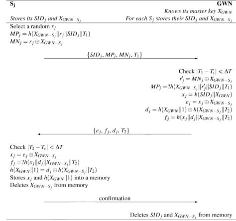
Figure 2. Sensor node registration phase of Farash et al.'s scheme [8].
