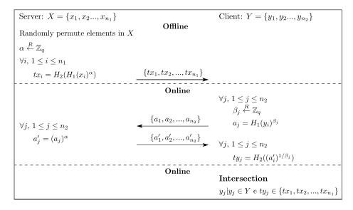
Fig. 1. Basic PSI protocol proposed in [5] that relaxes the security of the [23] to be secure against semi-honest adversaries.  $H_1$  and  $H_2$  are hash functions modeled as random oracles. [5, Adapted].
