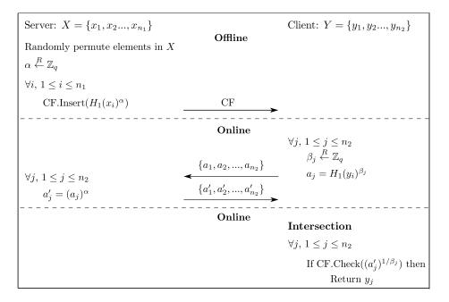
Fig. 2. Our optimized protocol combining the PSI protocol of Baldi *et al.* [5] with Cuckoo filter [41]. CF is a Cuckoo filter, CF.Insert is the insertion operation and CF.Check is the lookup operation, presented in Section 4.2.  $H_1$  is a hash function modeled as random oracles.
