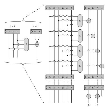
Fig. 10. Unbalanced Feistel network (left) and its TI (right).
