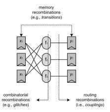
Fig. 3. Physical defaults for an exemplary TI (borrowed from [4]).
