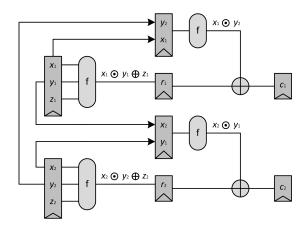
Fig. 2. Example of 2-share/2-cycle decomposition of a Toffoli gate.
