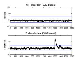
**Fig. 6.** Non-specific T-test results for a first-order TI of the PRESENT S-box tweaked so that the register storing  $x_1$  and  $y_1$  in Figure 3 is re-used with refreshing.
