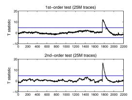
**Fig. 5.** Non-specific T-test results for a first-order TI of the PRESENT S-box tweaked so that the register storing  $x_1$  and  $y_1$  in Figure 3 is re-used without refreshing.
