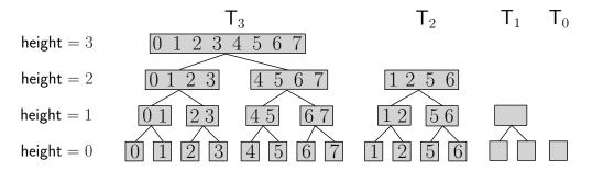
Figure 1: Hierarchy of range trees. Logically, data is divided into trees of exponentially increasing sizes. In each tree block, a parent super-block stores the contents of both its children. If a block appears in more than one tree, the smallest tree contains the freshest copy. The above figure shows the state of the data structure after two accesses (read,  $5, 2, \perp$ ) and (read,  $1, 2, \perp$ ).
