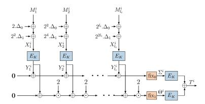
Figure 4.1: 1k-PMAC\_Plus Construction
