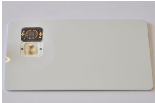
(a) SmartCafe Expert 6.0 chip removal
