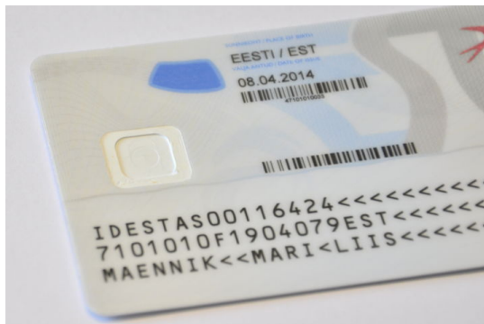
(f) ID card with chip removed
