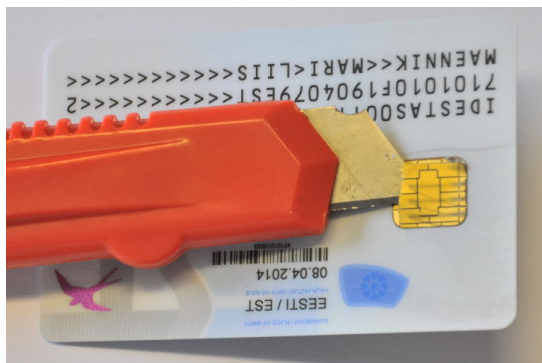
(c) ID card chip removal
