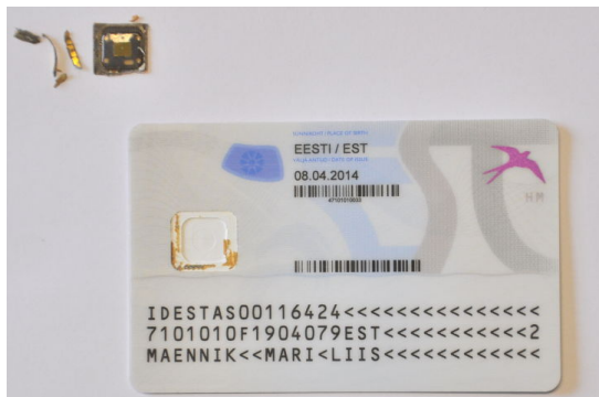
(e) ID card with chip glue residues
