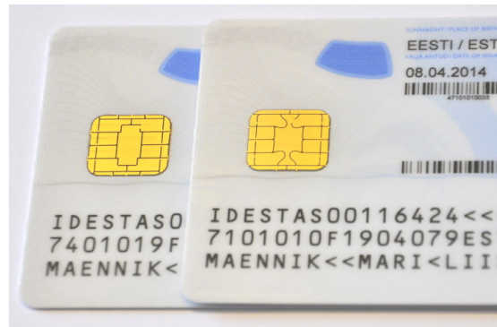
Fig. 3. Original vs. transplanted card
