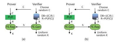
**Fig. 2.** Reproducible and uniformly distributed key from PUF. (a) Fuzzy Extractor. (b) Reverse Fuzzy Extractor.
