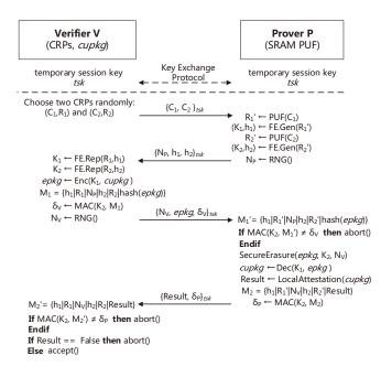
Fig. 3. Secure Code Update Protocol based on PUF
