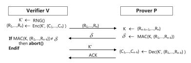
Fig. 1. Secure Code Update Protocol based on PoSE
