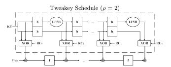
Fig. 1. TWEAKEY framework for Deoxys-BC.
