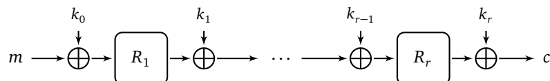
Figure 1: Key-alternating construction for r rounds, using unkeyed round permutations R_1 to R_r . In practical instantiations, the round keys k_i are typically derived from a master key by some key schedule.
