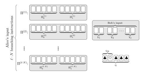
**Fig. 6.** Overview of the branching program construction. Alice's input is the branching program  $((j^{(i)}, \pi_0^{(i)}, \pi_1^{(i)}))_{1 \leq i \leq N} \in (\{1, \dots, \ell\} \times S_5 \times S_5)^N$  in normalized form.
