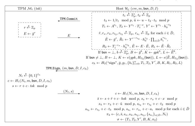
**Fig. 3.** The sign protocol of DAA<sub>0PT</sub>. For the case that  $bsn \neq \bot$ , *B* is set as  $\bot$ , as  $e(\bar{g}, H_{\mathbb{G}_2}(bsn))$  can be computed offline by the verifier. The elements marked in the dashed box can be computed offline by the TPM and host. Again, TPM.Commit and TPM.Sign represent the TPM requests rather than real TPM 2.0 commands.
