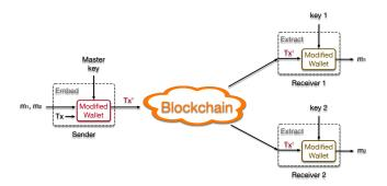
Fig. 11. Attack scenario 1: Covert broadcast communication.
