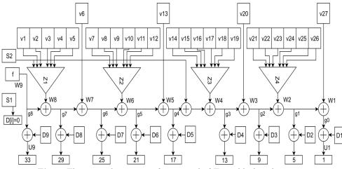
Fig. 2. The internal structure of one round of T-310 block cipher.
