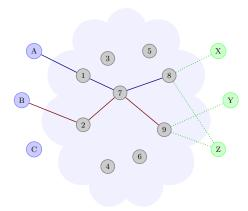
Fig. 1: Onion routing in a nutshell. Nodes A, B, and C are the onion proxies; nodes 1 to 9 are the onion routers making up the network; finally nodes X, Y, and Z are the destinations. User A created the dark blue circuit 1–7–8, using exit node 8 to communicate with destinations X and Z, whereas user B created the dark red circuit 2–7–9 and using its exit node 9 to communicate with destinations Y and Z.
