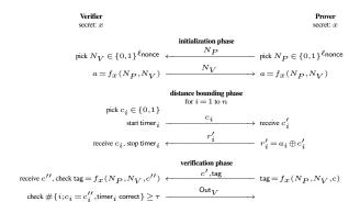
**Fig. 1.** The DB3 Distance-Bounding Protocol with q = 2.
