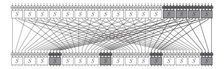
Fig. 3. work model of super S-box in PRESENT
