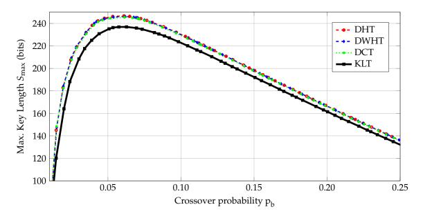
**Figure 3.** The maximum key lengths  $S_{\text{max}}$  for  $8 \times 8$  RO arrays.
