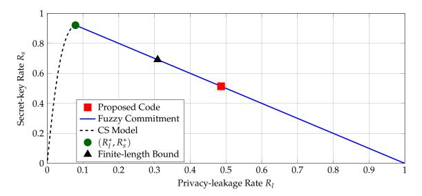
**Figure 7.** The operation point of the proposed BCH code C(255, 131, 37), regions of achievable rate pairs according to (5) and (6), the maximum secret-key rate point, and a finite-length bound for N = 255 bits,  $P_B = 10^{-9}$ , and BSC(0.0097).
