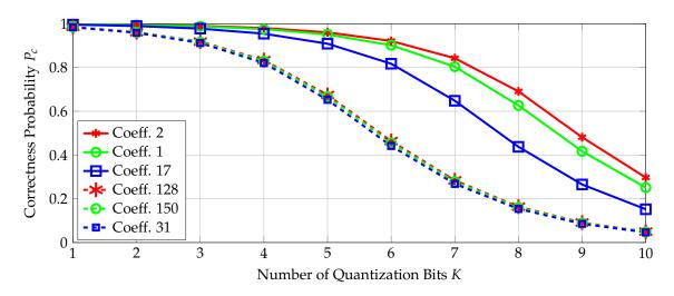
Figure 6. The correctness probabilities for transform coefficients.
