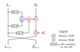
Figure 5: Schematic of one round of SIMON block cipher.
