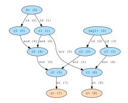
Figure 9: Updated graph generated by TADA after two successful attacks on vulnerable instruction 4 of example cipher  $\mathcal{F}_{ex}$  in Table 2.
