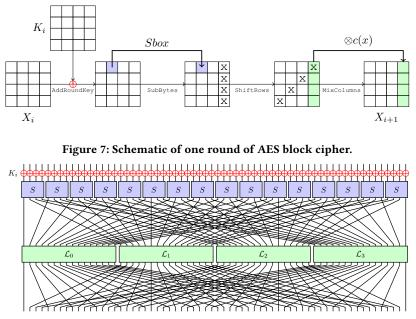
Figure 8: Schematic of one round of PRIDE block cipher.
