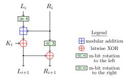
Figure 6: Schematic of one round of SPECK block cipher.
