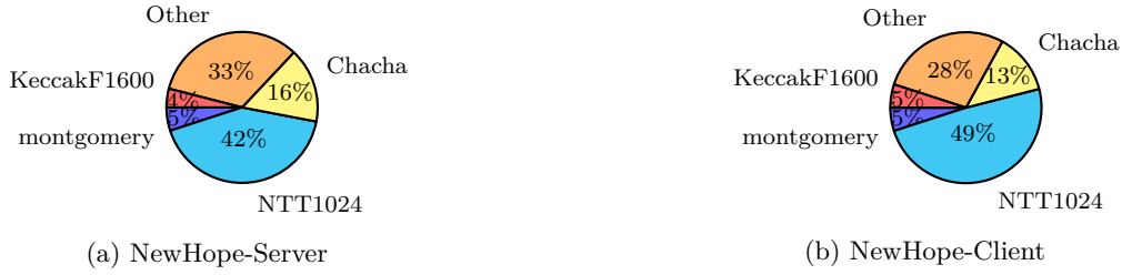
Figure 1: Breakdown of NewHope into kernels in terms of (exclusive) CPU cycles (kernels with less than 4% are grouped into Other ).
