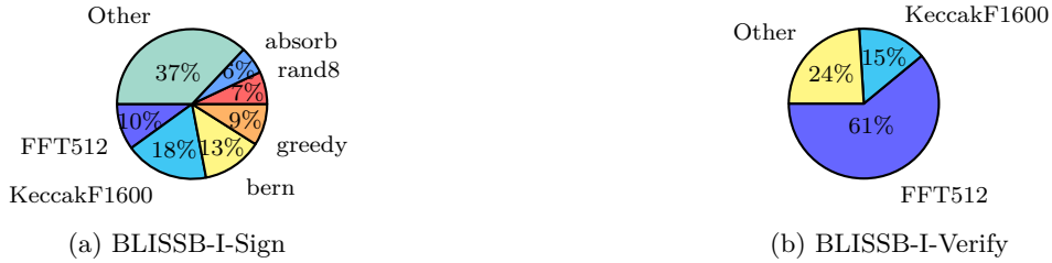
Figure 2: Breakdown of BLISSB-I into kernels in terms of (exclusive) CPU cycles (kernels with less than 4% are grouped into Other ).
