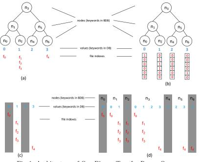
Fig. 1: Architecture of Our Binary Tree for Range Query
