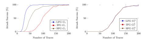
Fig. 6. Graph combination methods using Graphs  $G_1$  and  $G_1^A$ , SNR  $2^{-6}$
