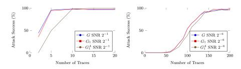
Fig. 7. Reduced Graph comparison using SNRs  $2^{-1}$  and  $2^{-6}$  respectively
