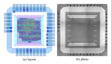
Fig. 5: ASIC prototype with 6 cores in 150 nm CMOS.
