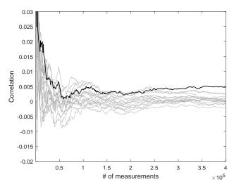
Fig. 18: CPA on Hamming weight of 12-bit F-box output for a measurement interval of 1 ms at a supply voltage of 1.98 V and a temperature of  $90 \text{ }^{\circ}\text{C}$
