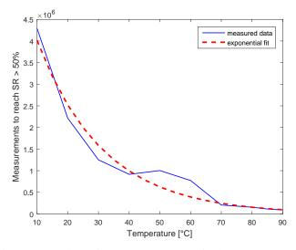
Fig. 10: Number of measurements required to overcome a success rate of 50 % for temperatures between  $10 \,^{\circ}\text{C}$  and  $90 \,^{\circ}\text{C}$
