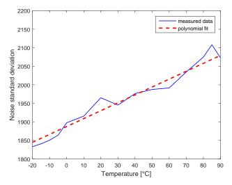
Fig. 9: Estimated noise standard deviation for temperatures between -20 °C and 90 °C
