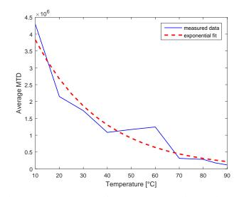
Fig. 11: Average number of measurements required to disclose the correct key candidate for temperatures between  $10 \,^{\circ}C$  and  $90 \,^{\circ}C$
