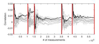
Fig. 8: Visual depiction of our technique to use disjoint subsets of one large set of traces to disclose the key multiple times. The shown MTD values (achieved for  $90 \,^{\circ}$ C,  $1.98 \,$ V,  $10 \,$ ms) from left to right are 85 000, 28 000, 181 000, 59 000, 143 000.
