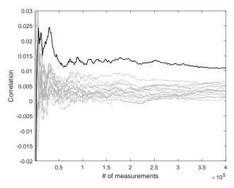
Fig. 17: CPA on Hamming weight of 12-bit F-box output for a measurement interval of 200 ms at a supply voltage of 1.98 V and a temperature of  $90 \text{ }^{\circ}\text{C}$
