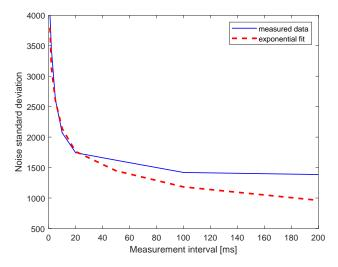
Fig. 15: Estimated noise standard deviation for measurement intervals between 1 ms and 200 ms at a supply voltage of 1.98 V and a temperature of  $90 \text{ }^{\circ}\text{C}$
