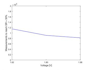
Fig. 13: Number of measurements required to overcome a success rate of 50 % for supply voltages between 1.62 V and 1.98 V and temperature of 90 °C
