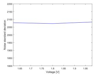
Fig. 12: Estimated noise standard deviation for supply voltages between 1.62 V and 1.98 V and temperature of  $90 \,^{\circ}\text{C}$
