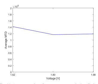
Fig. 14: Average number of measurements required to disclose the correct key candidate for supply voltages between 1.62 V and 1.98 V and temperature of  $90 \text{ }^{\circ}\text{C}$
