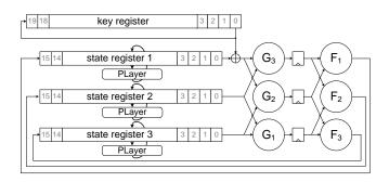
Fig. 6: Nibble-serial architecture of the PRESENT-80 threshold implementation core.
