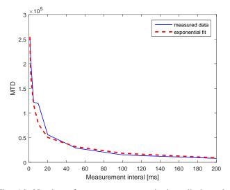
Fig. 16: Number of measurements required to disclose the correct key candidate for measurement intervals between  $1\,\rm{ms}$  and  $200\,\rm{ms}$  at a supply voltage of  $1.98\,\rm{V}$  and a temperature of  $90\,^{\circ}\rm{C}$
