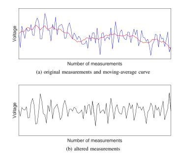
Fig. 7: Illustration of the post-processing technique for 100 exemplary measurements at 20 °C, 1.8 V, measurement interval of 10 ms and window-size of 8.
