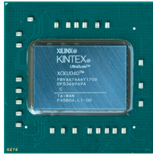
Figure 5: Image of a Xilinx Ultrascale XCKU040-1FBVA676 device in a flip-chip BGA package [AVN18]. The exposed silicon backside of the die can be seen in the middle of the package.
