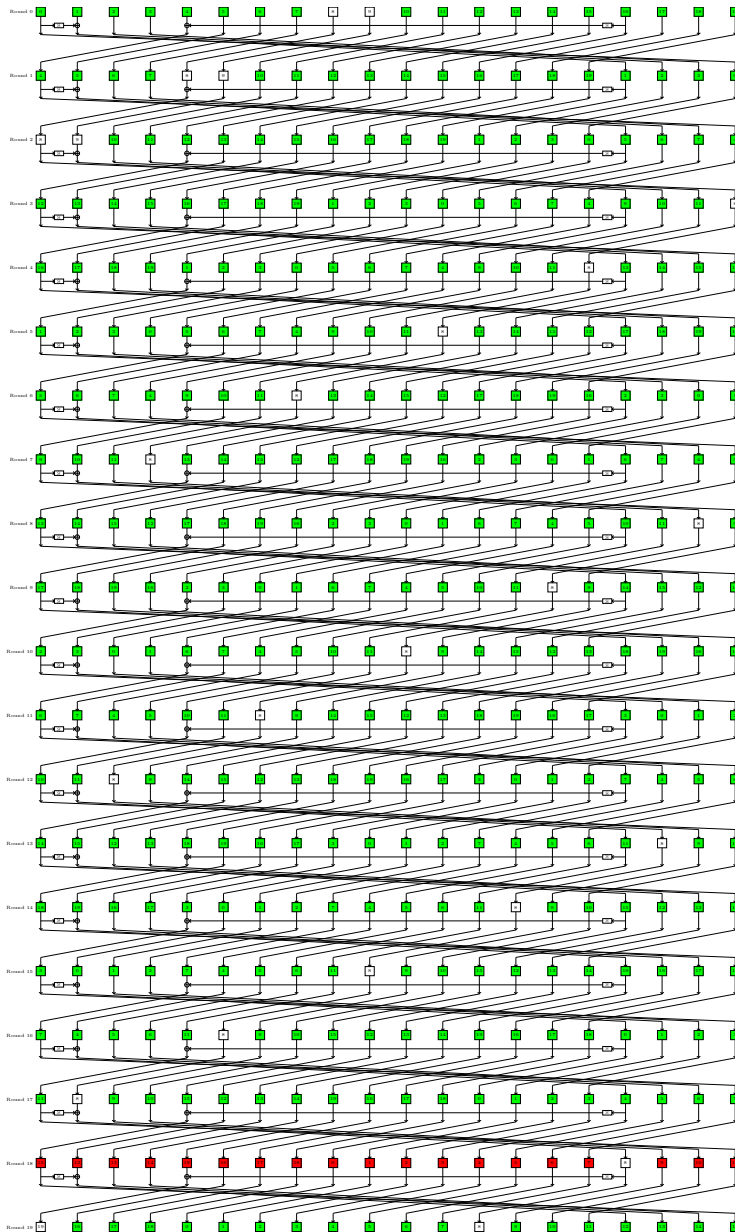
Fig. 27: A illustration that if we know the nibbles marked with red in round 18 of the key schedule algorithm of TWINE, we can derive the values of all the nibbles marked with green in the other rounds. The reader can verify that all the nibbles marked with orange in Fig. 26 are included in the colored nibbles of this figure.
