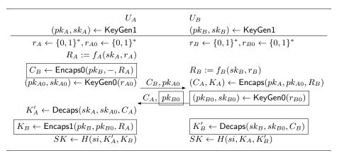
**Fig. 3.** AKE<sub>ro-pkic</sub> from PKIC [OW-CCA, OW-CPA] secure 2KEM. Here  $si = (U_A, U_B, pk_A, pk_B, C_B, pk_{A0}, C_A, pk_{B0})$ . The boxed argument is the difference with AKE
